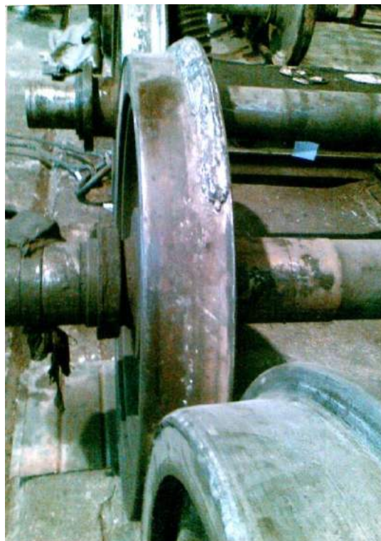
Fig.5 – Type of threadbare wheel pair
